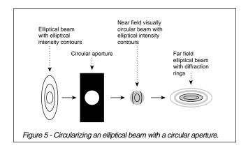
transmitted beam power is significantly reduced. However such truncation does suggest one simple method of circularizing a diode beam.
