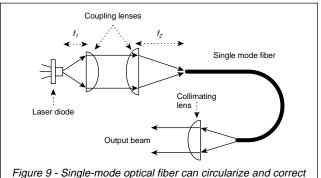
Figure 9 - Singie-mode optical fiber can circularize and correct astigmatism of a laser diode beam.
