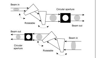
Figure 8 - A pair of anamorphic prisms can enlarge or reduce the beam size along one axis while keeping the beam size in the perpendicular direction unchanged.
