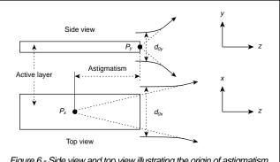
Figure 6 - Side view and top view illustrating the origin of astigmatism.
