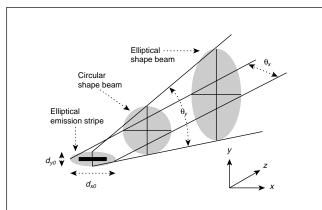
Figure 2 - The output beam from the emission stripe diverges rapidly and the beam shape changes as the beam propagates.
