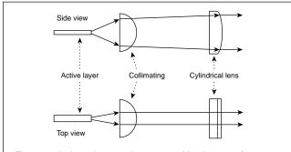
Figure 7 -Astigmatism can be corrected by the use of a cylindrical lens with long focal length.
