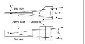
Figure 10 - An appropriate micro-cylindrical lens positioned properly can circularize an elliptical beam and correct the beam astigmatism.
