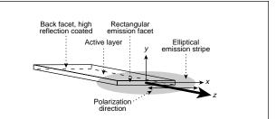
Figure 1 - Laser diodes have a thin active layer with a rectangular cross section. The emission stripe at one end of the active layer has an elliptical cross section and is larger than the cross section of the active layer. The drawing is not to scale.
