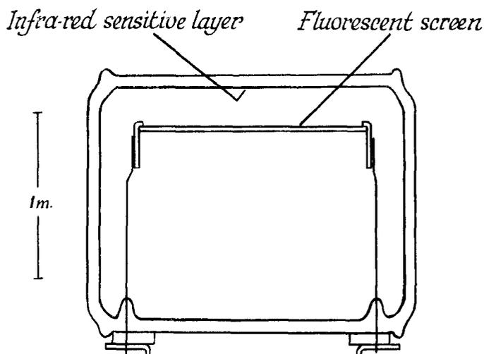
Fig 1. Diagram of infra-red image-converter tube
