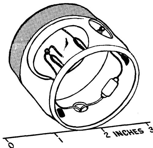
Fig 2. Infra-red image-converter tube
