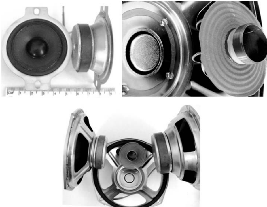
FIGURE 4.30 Speakers as limited-displacement permanent-magnet DC actuators.
